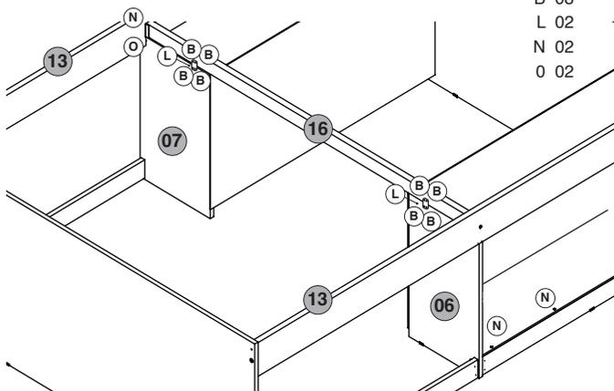
FIXE O SARRAFO CENTRAL (16) USANDO SUPORTE DE SARRAFO (O) E PARAFUSOS (N). FIXE A FACES DAS DIVISÓRIAS MENORES DIREITA (6) E ESQUERDA (07) NA FACE DO SARRAFO USANDO A CHAPINHA (L) E OS PARAFUSOS (B), COMO MOSTRADO NA IMAGEM.
